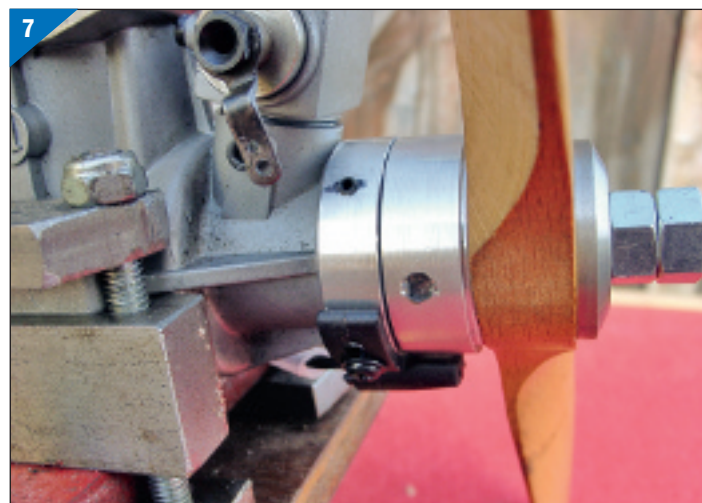
Modified ASP91 2-stroke. One aluminium ring has been used to house the magnet and another to carry the sensor bracket.
